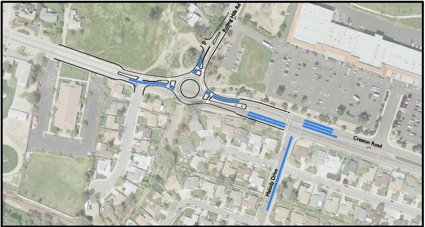
Queues with Roundabout at Rolling Hills Road
